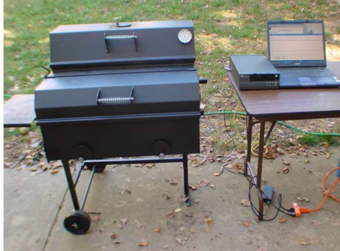
Figure 1. Overview of the test set-up, showing smoker, computer, and data acquisition system.
